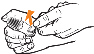
Pulling the mouthpiece from the cooling unit cap
