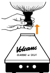
Remove Valve Balloon with Filling Chamber
