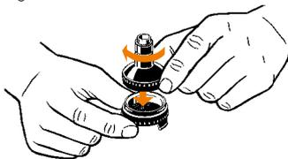
Screw on Filling Chamber Cap
