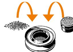
*Fill the Filling Chamber Reducer with ground plant material directly or with a filled Dosing Capsule*
