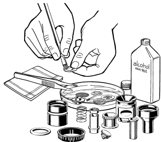
Manual cleaning with isopropyl alcohol (70 %) or detergent
