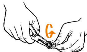
Disassembling the Filling Chamber Insert
