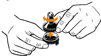
Screw on Filling Chamber Cap
