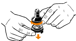
Screw on Filling Chamber Cap
