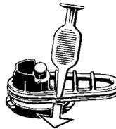
Lever out the large Base Seal Ring with the Filling Chamber Tool.
