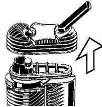
Pull the Cooling Unit Cap off the Vaporizer.
