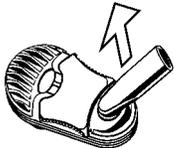
Pull the Mouthpiece out of the Cooling Unit Cap.
