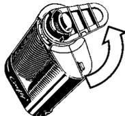
Unscrew the Cooling Unit Base from the Vaporizer.
