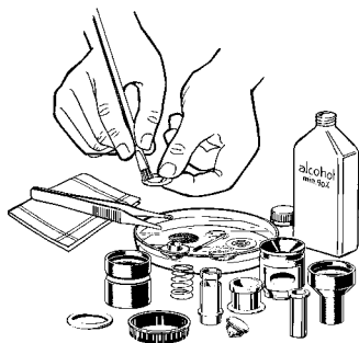
11. Manual cleaning with alcohol (min. 90%), also dishwasher safe
