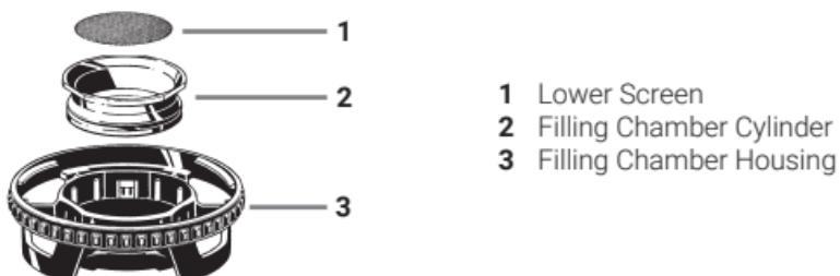
**Disassembling the Filling Chamber**
