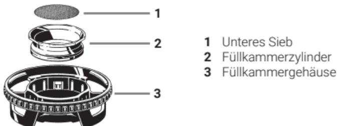
**Zerlegen der Füllkammer**
