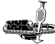
Lever out the large Base Seal Ring with the Filling Chamber Tool.
